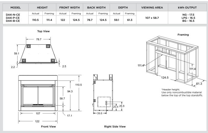
Dimensions above are in centimeters and for reference only. We recommend measuring individual units at installation. Assumes the use of 1.3cm gyprock. Refer to installation manual for detailed specifications on installing this product. Heat & Glo reserves the right to update units periodically. The flame and ember appearance may vary based on the type of fuel burned. Photos in this brochure may vary in color and dimension [size] from the actual product.
